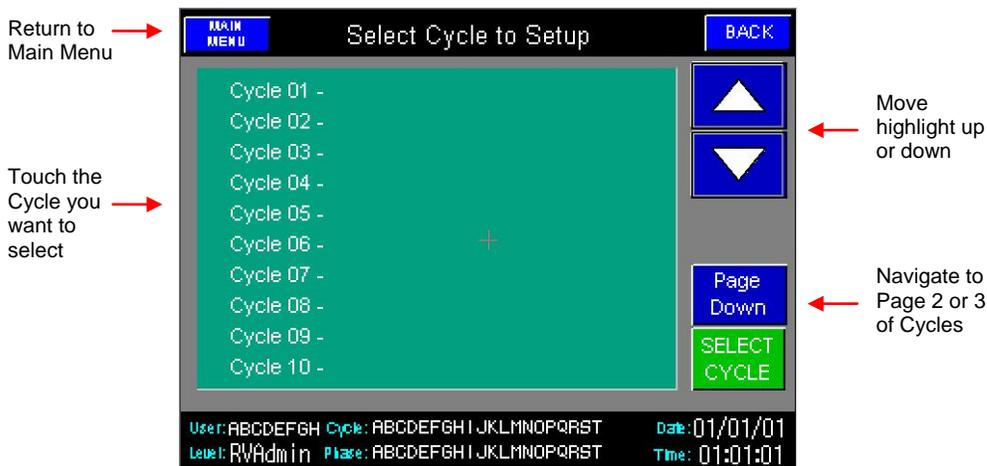
To select a cycle to setup, touch the cycle you want to select, or use the arrow buttons to move the screen highlight to the cycle you would like to select. You can Page Down for more options, the system holds a total of 30 cycles. When you have select the cycle you would like to setup, press the SELECT CYCLE button.
