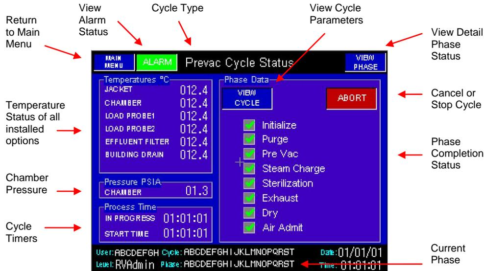
The Phase Data box provides a list of the phases required for the type of cycle you are running. A green  indicates the phase has been completed, a yellow  in check box indicates the phase is not completed. The phase currently running is displayed in the center bottom of the status bar.
