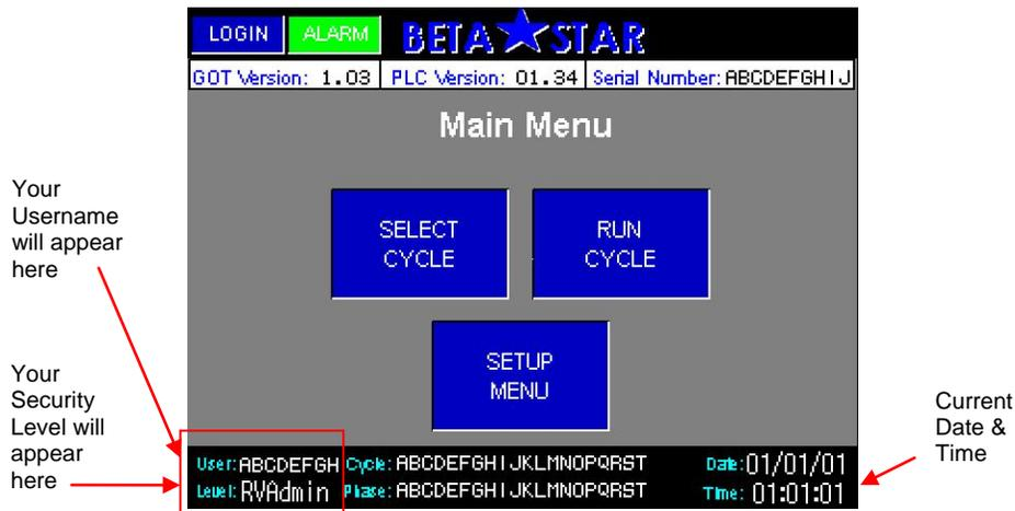
From any screen that contains the status bar, you can login or logout by pressing the area of the status bar that contains the User name and Security Level. See red box above.
