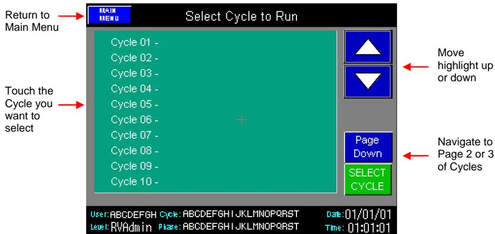
To select a cycle, touch the cycle you want to select, or use the arrow buttons to move the screen highlight to the cycle you would like to select, then press the SELECT CYCLE button. You can Page Down for more options, the system holds a total of 30 cycles.
