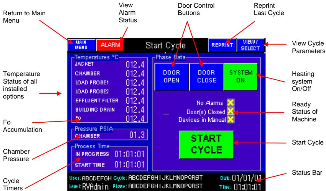
To start a cycle, the system must be in the ready state. This means there can be no active alarms, the door(s) are closed, and the system is in automatic mode. The Ready Status is displayed above by the 3 green , if the system was not ready, one or more of the check marks would be a yellow .
