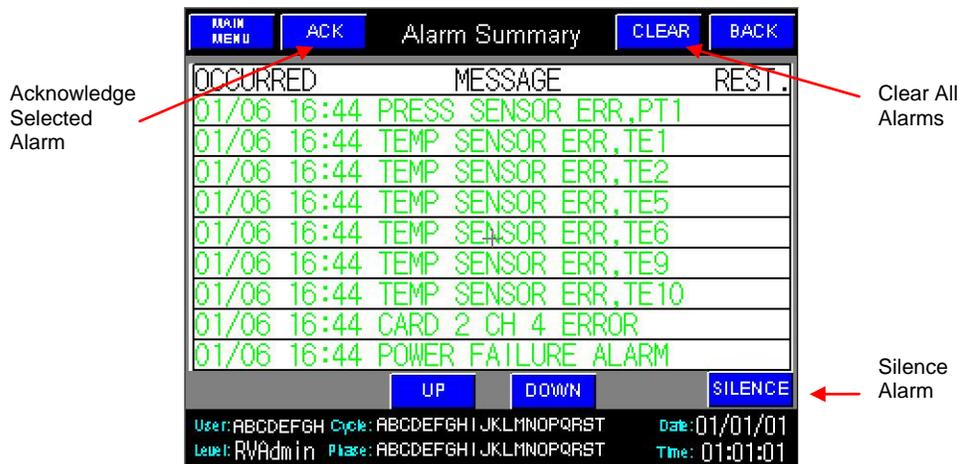
You can acknowledge an alarm by pressing the alarm description you want to acknowledge and then pressing the ACK button.
