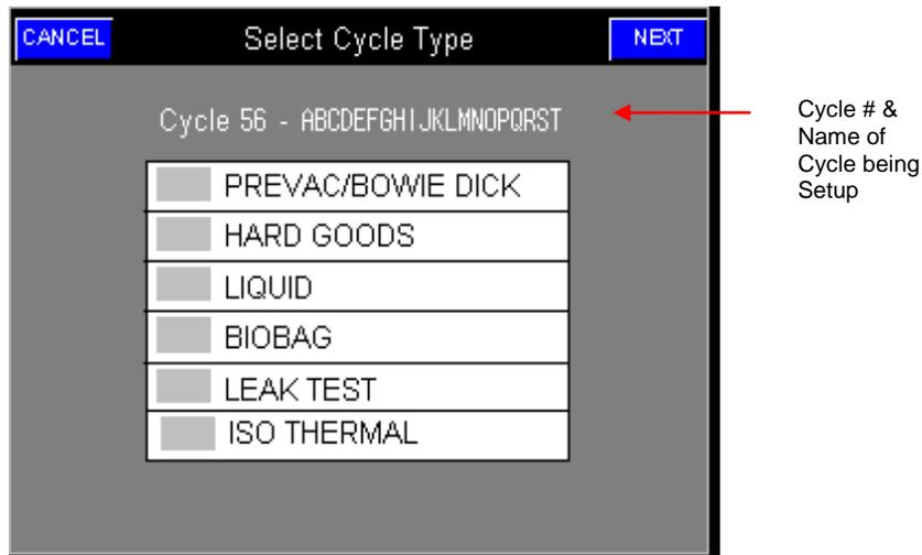
Press one of the five cycle types to select the type of cycle you want to setup. (See the Cycle Definitions section of the manual for detailed descriptions of each cycle type.) The Cycle Type you selected will now be highlighted; you can change your selection by pressing one of the other types. When you have completed your selection press the NEXT button, this will bring up the Cycle Setup screen below.
