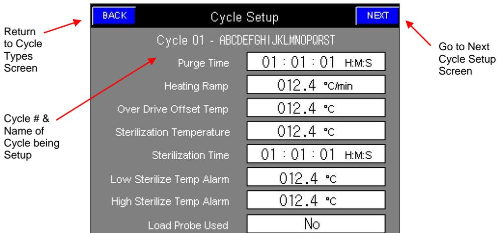
From the Cycle Setup screen you can return to the Select Cycle Type screen using the back button or go forward to the next Cycle Setup screen. Each white box represents a configurable cycle parameter, to edit a parameter, press on the white box of the parameter you would like to change. If the value you want to change is a yes/no value, pressing the box will toggle the values.
