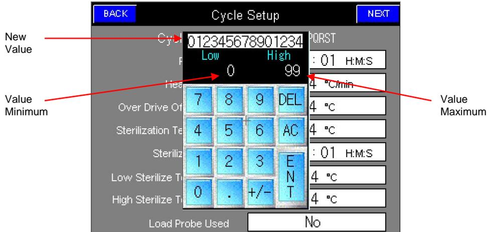
On the keyboard you will see a Low value and a High value; these are the upper and lower limits of the parameter you selected. You must enter a value between the Minimum and Maximum. To enter the new value, simply press the numeric keys on the keyboard, when complete press the ENT key to enter the new value into the parameter you selected.
